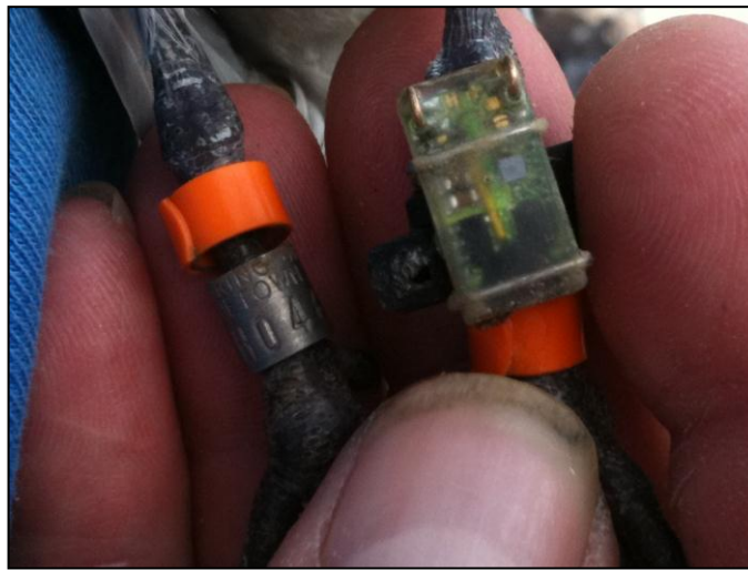
Figure 3. A Sooty Tern carrying a geolocator attached to a leg ring. (Photo: Simon Croson).
